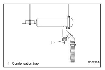
Figure 5-3 Condensation Trap
